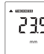
In a well coupling measurement
